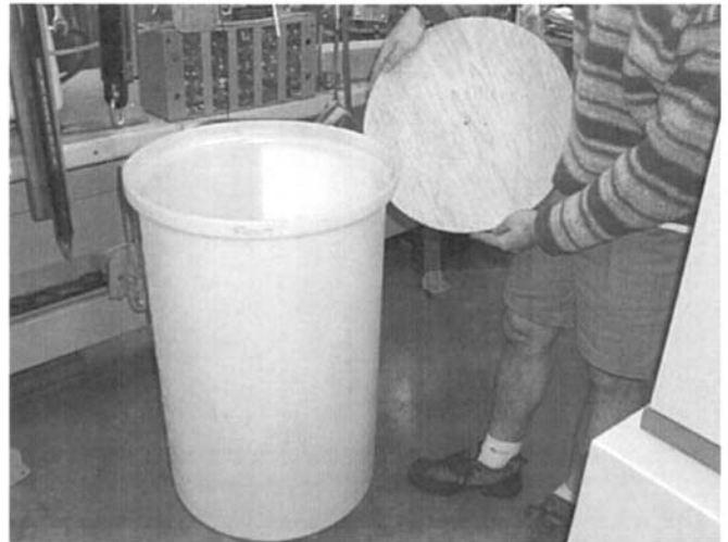
FIG. 2 Typical 18-in. Diameter Cylinder: Measurement Tool in Hand
